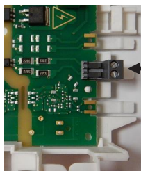
I1 Photovoltaic connection contact 230V ~
